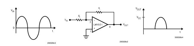
FIGURE 3. Half-Wave Rectifier with Rail-To-Ground Output Swing Referenced to Ground
