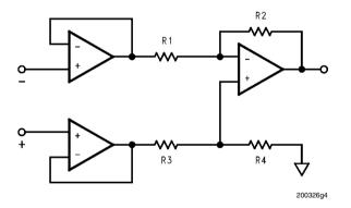
FIGURE 5. Rail-to-rail Instrumentation Amplifier
